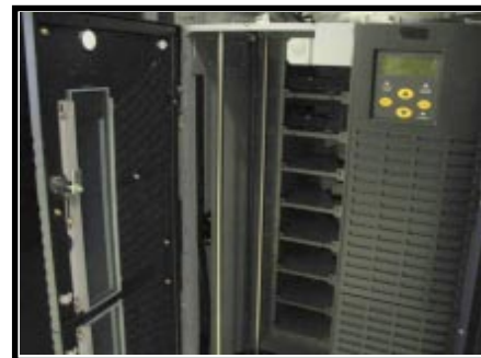
WILTEC Model 510-L LTO1/2/3/4 Dual Magazine capacity to 80 cartridges/load are easy and fast to load/reload.
